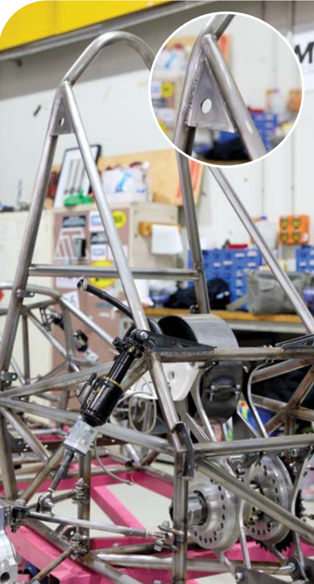
Formula SAE space frame fabricated from UltraTube RS by the University of Waikato’s WESMO team.
